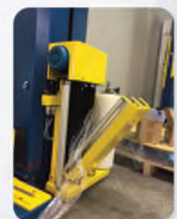
FILM CARRIAGE with POWER PRE-STRETCH (200 % FIXED RATIO)
